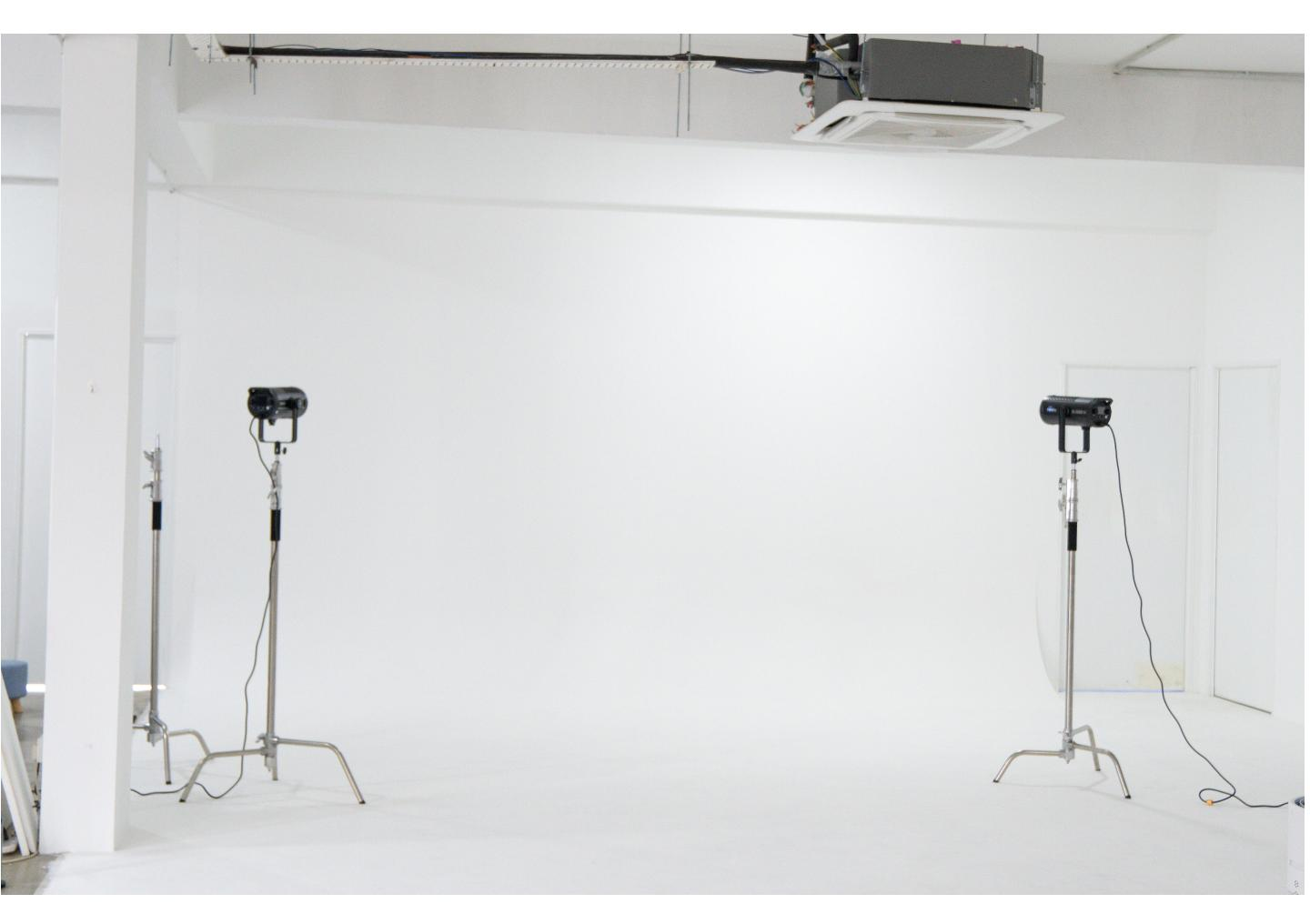
An infinity wall, also known as an infinity curve or cyclorama, is a curved wall typically used in photography, videography, and film production. It's designed to create a seamless, continuous background without any visible corners or edges, giving the illusion of infinite space.
